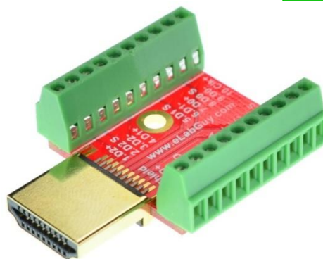
Figure 4: HDMI-AM-BO-V1B with terminal blocks
