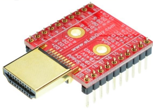
Figure 3: HDMI-AM-BO-V1B with headers
